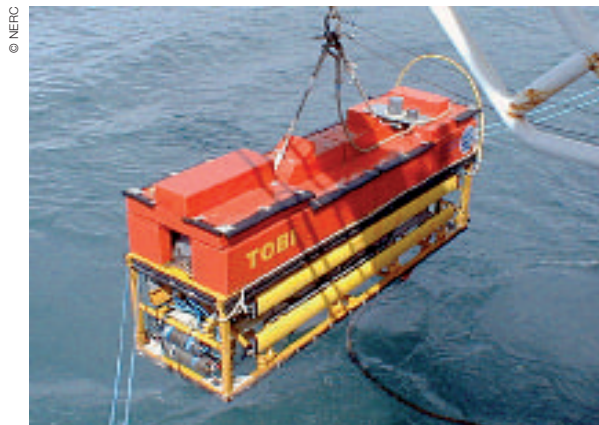
TOBI, a seafloor mapping system
